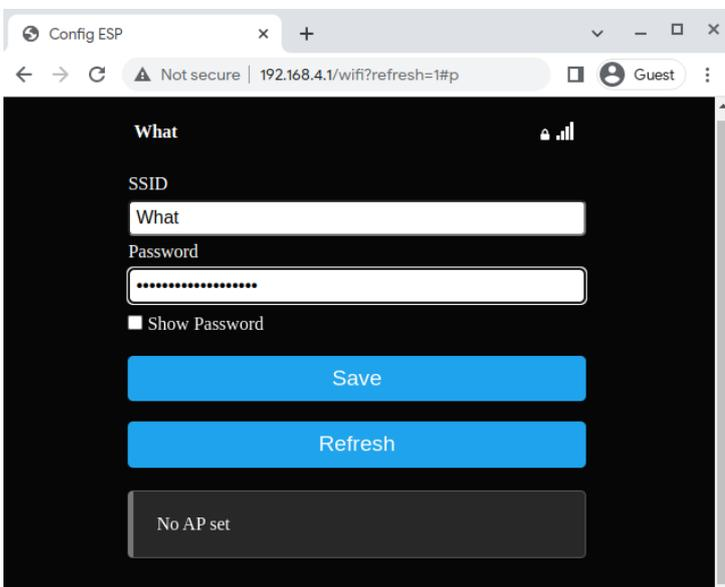
If your wifi network doesn't show in the scan results, your NodeMCU might not support it. Please ensure the wifi network has 2.4 GHz support and your NodeMCU is close enough to the router.
